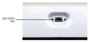
2 Press the sync button on the bottom of your keyboard until your computer's RF sync indicator flashes. Your keyboard is now synced with your computer.
